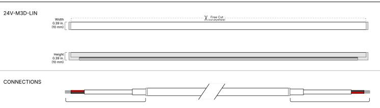
96 in. White Bare Lead 20/2 AWG UL 2464 Wire with Strain Relief
